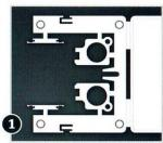
Snap off the 2x keys and 2x cable hole covers from the back of the SocketLoc. Add foam pads to the indicated areas on the back surface.
