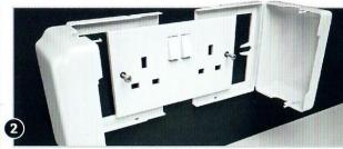
Loosen screws on your plug socket by approximately 4mm. Slide the backplate in behind the socket from either the left or right hand side of the socket and ensure the screw locator lug fits around the screw. Ensure that each backplate overlaps each other at the top and the bottom. Before fully tightening the screws push the 2 top covers together without snapping them into place, so that they are almost touching each other, then tighten the screws fully.
